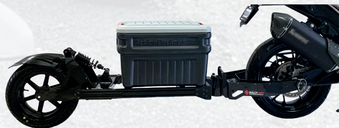
Short trailer equipped with a 90L plastic bin
