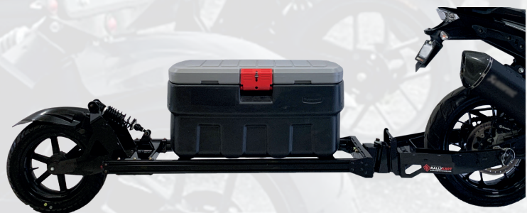
Trailer equipped with a 140L plastic bin
